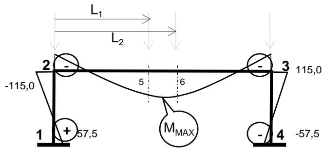
$$M_5 = -M_2 + Q_2 \times L_1 - q \times L_1^2 / 2 = -115,0 + 109,9 \times 6,90 - 9,50 \times 6,90^2 / 2 = \underline{417,2 \text{ tm}}$$
