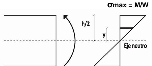
**DIAGRAMA DE TENSIONES PARA UN MATERIAL HOMOGÉNEO**
